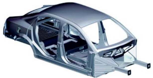
Figure 5: ULSAB-AVC Bodies-In-White; top shows C-Class (mass = 202 kg/445 lbs.); bottom shows PNGV-Class (mass = 218 kg/481 lbs.)
