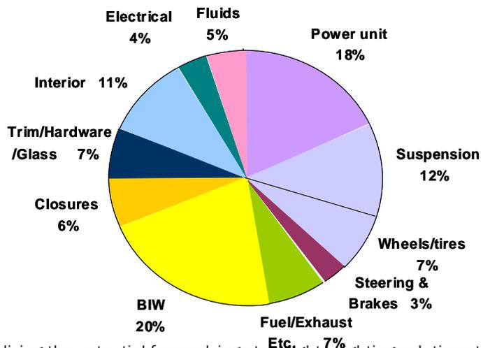
Realizing the potential for applying steel lightweighting solutions to suspension systems, the ULSAS consortium undertook a comprehensive study focusing solely on this area.
