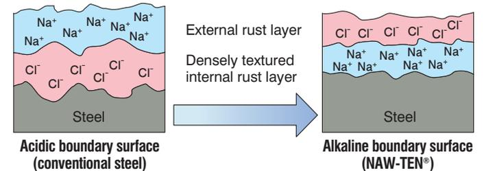
The rust layer is composed of two structures, and when the internal rust layer is stable and solid, corrosion ceases to develop.
